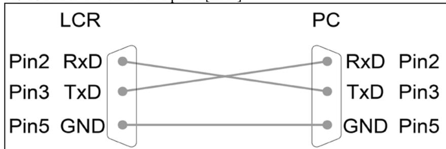
The RS-232 serial interface can be interconnected with a serial interface of a controller (eg PC or IP) via a 2-3 crossed DB-9 cable.
