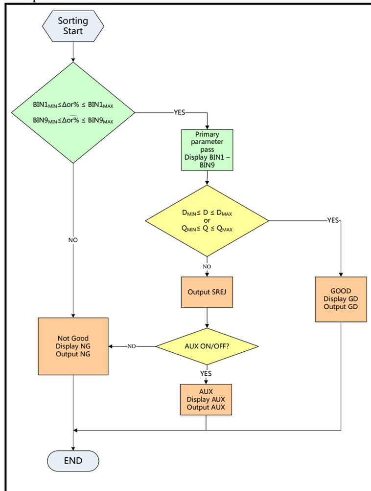
■ Procedure for setting the comparator function [COMP]
