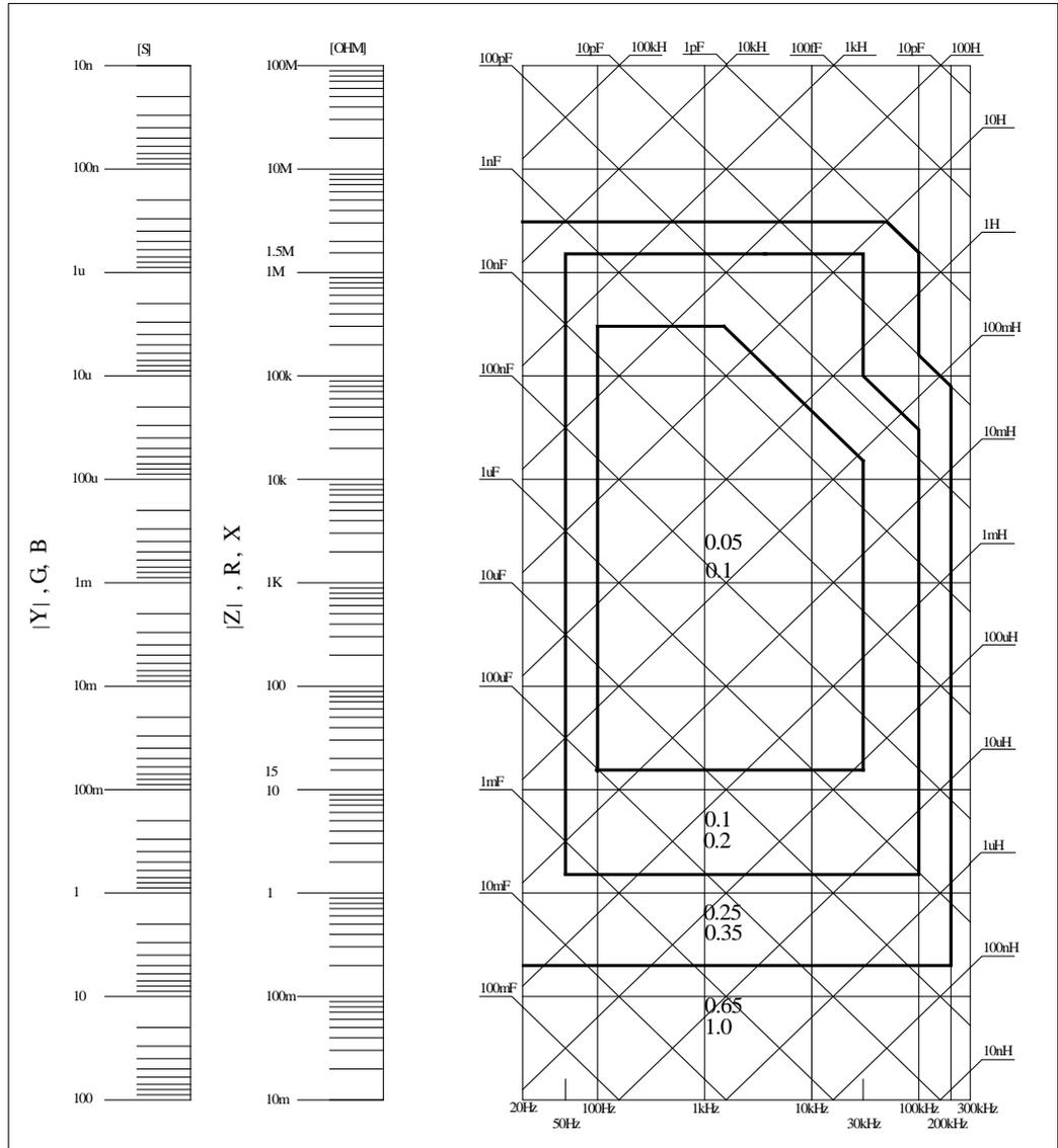
Figure 13-1 In the basic measurement accuracy, select a smaller value on the boundary line.
