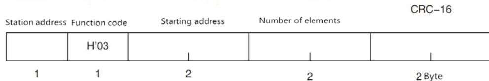
The function code for reading multiple registers is 0x03.
